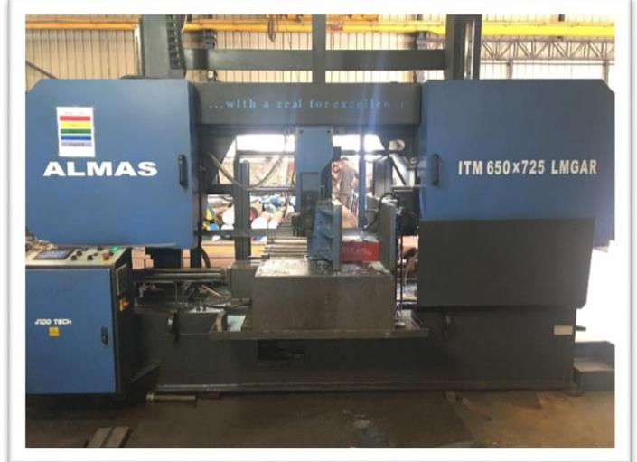
3. Full Automatic Bandsaw Machine- Diameter 70-300mm
