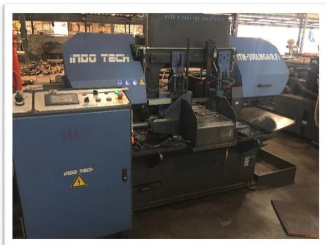
6. Full Automatic Bandsaw Machine- Diameter 100-300mm
