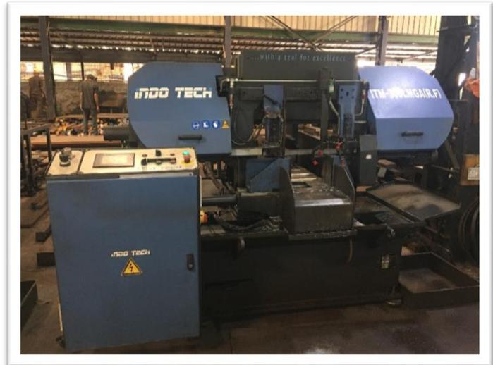
7. Full Automatic Bandsaw Machine- Diameter 100-300mm
