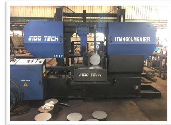
5. Full Automatic Bandsaw Machine- Diameter 100-300mm
