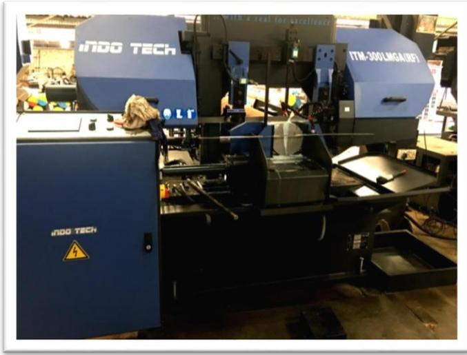
8. Full Automatic Bandsaw Machine- Diameter 100-300mm
