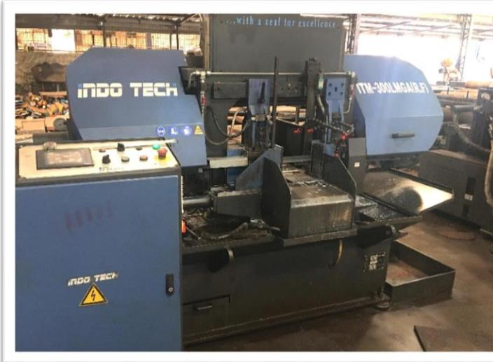
4. Full Automatic Bandsaw Machine- Diameter 70-500mm
